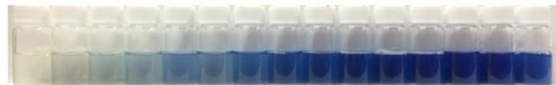
Figure 3. Dispersion liquid of poly-DCHD nanocrystal prepared by adding Triton X-100 under different retention times (from left: 1,2,3,4, 8, 12, 16, 20, 24, 28, 32, 36, 40, 44 minute)
