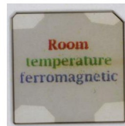
Fig. 1. Photograph of semitransparent, electrically conducting, room temperature ferromagnetic, and chemically durable cobalt-doped TiO 2 thin film.
